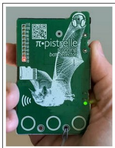
π-pistrelle handheld bat detector / 384kHz full-spectrum recorder / 384kHz USB microphone : APPROX £20 BUILD COST
