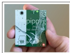
pippy static bat detector with 384kHz full-spectrum recording. Runs for up to 7 days powered by 3x AA rechargeable batteries, records to microSD card : APPROX £15 BUILD COST
